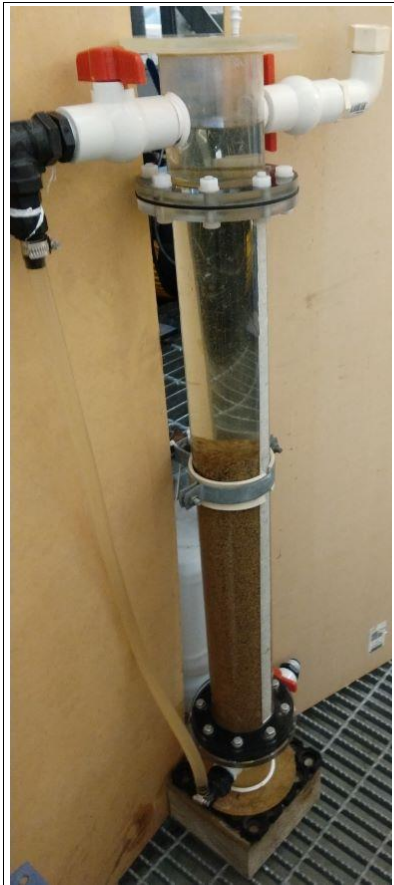
Figure 9: Stage 2 column contactor with fixed bed Ardmore apatite
